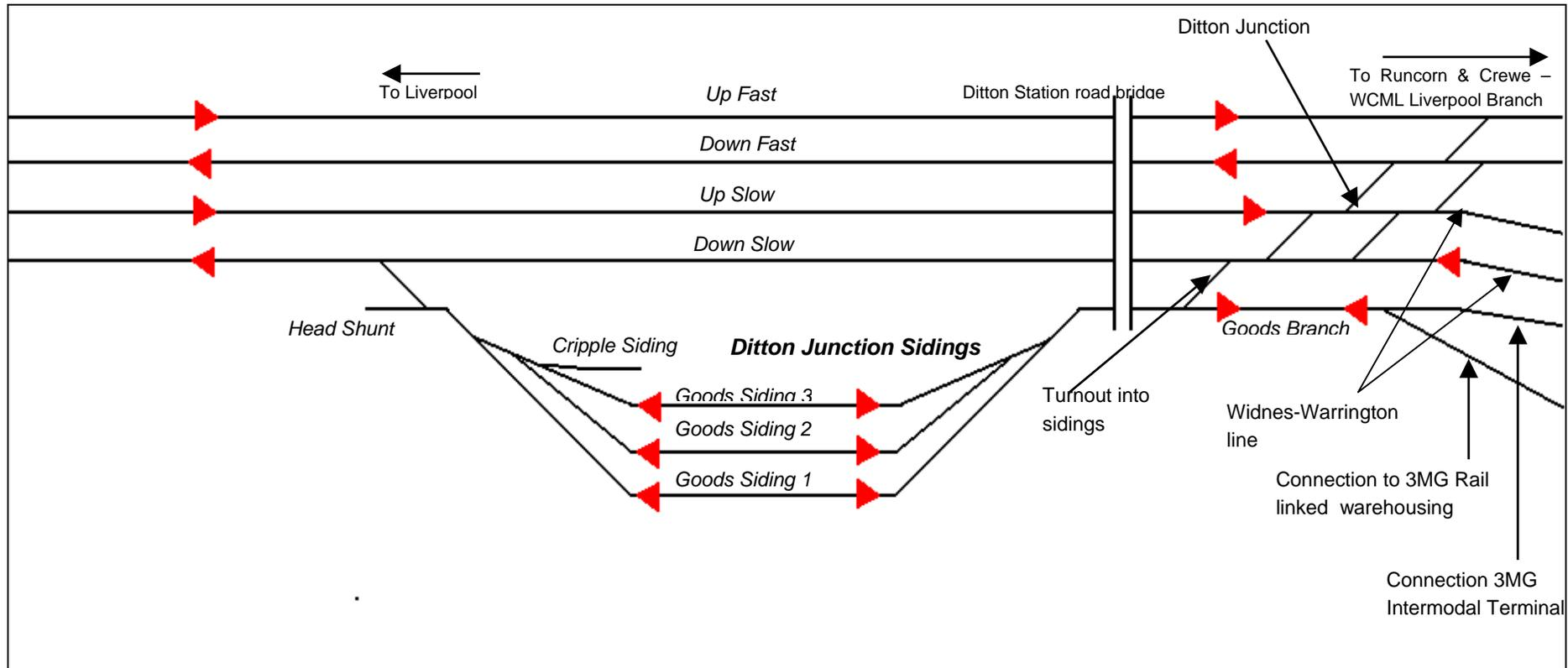
**Not to Scale. The red arrows indicate direction of signalling on each line. Arrows pointing in opposite directions on a line indicates bi-directional signalling.**
