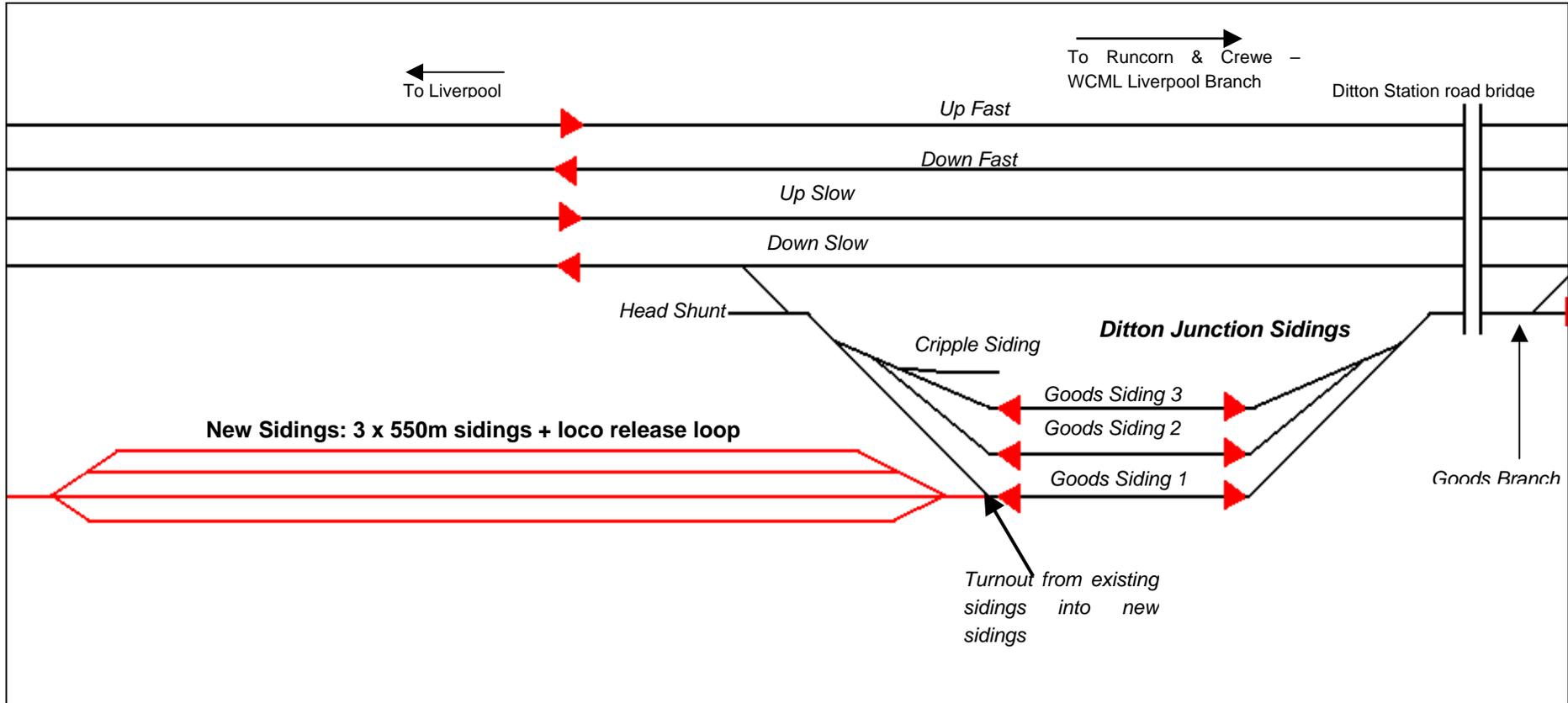
**Not to Scale. The red arrows indicate the direction of signalling on each line. Arrows pointing in opposite directions on a line indicates bi-directional signalling.**
